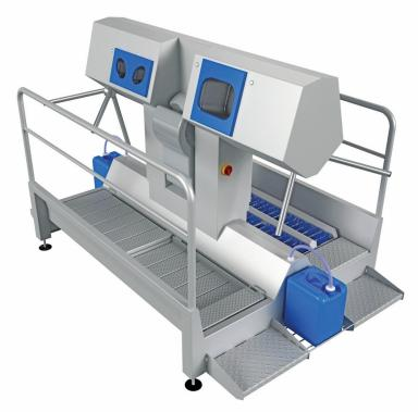
This Combi Double Hygiene Station has the perfectly controlled entrance and exit. During entry, the soles of the boots and the hands are disinfected by the station. The soles are cleaned and hands are disinfected again. Turnstile is released once disinfection is completed.
